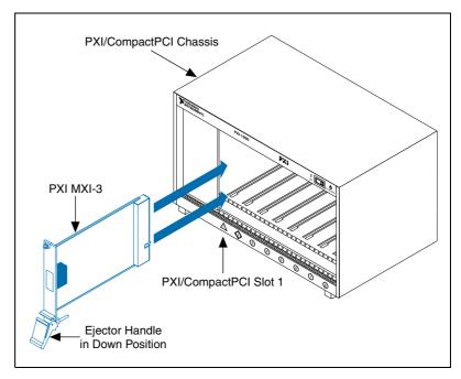
Figure 2-2. PXI MXI-3 Before Installation as Secondary
